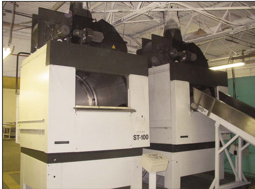
The two ST-100 Dryers at Resorts Laundry and Linen Services collectively dry 510 pounds of terry in 20 minutes.
